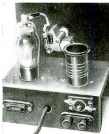
Rear view of the 1-tube Oscillodyne which has been made "all electric," thanks to the 12A7-type tube used, one element of which serves as the regenerative detector and the other element as a half-wave rectifier. This is essentially a headphone job.
