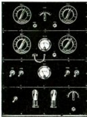
General appearance of the finished Rack and Panel Transmitter, the first unit of which is here described.
