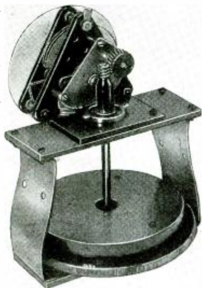
Photos, above and at right, show close-ups of the free wheeling dial and condenser as worked out by the author, and which provide rapid tuning with the equivalent of "band-spread."
